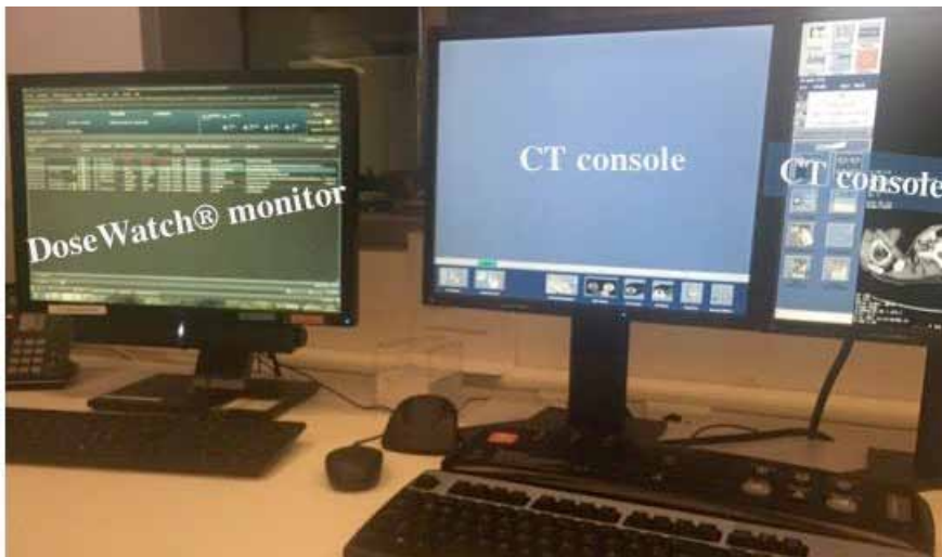
FIGURE 1. Placing the computer with the dose management software next to the CT console stimulates active involvement and collaboration by the CT technologists. DoseWatch is a GE Healthcare product and is a dose management solution designed to automatically collect and analyze patient radiation and iodine exposure in multi-modality and multi-vendor imaging environments.
